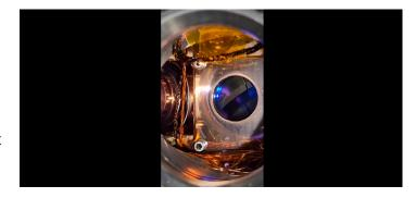
**Video 1:** The 2.5-second-long experimental cycle involves a green laser that cools and traps the atoms before the radiation shield is shifted to the closed position. The atoms are then excited by the clock laser (not visible) for about half a second, and then the shield is opened, and the atoms' state is determined with another laser (not visible), whereupon the cycle restarts.
